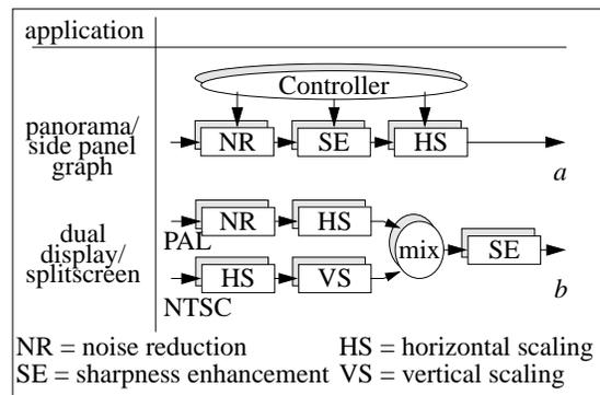
Figure 2: Same coprocessors used in different configurations and settings (50 Hz system).
