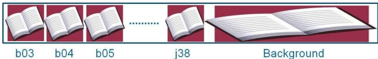
Figure 4. Illustration of the modular codebook: a concatenation of multiple smaller codebooks representing the different sign classes together with a larger codebook representing false detections.
