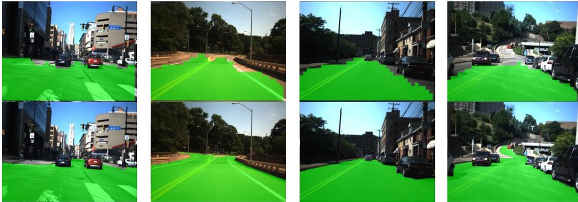
Fig. 4. Example results of our online self-supervised road detection system using a RBF-SVM with the HS144 feature space. Classification results are shown in top row and ground truth labels are shown in bottom row.
