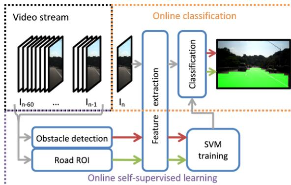
Fig. 1. Overview of the integrated road and obstacle detection system.
