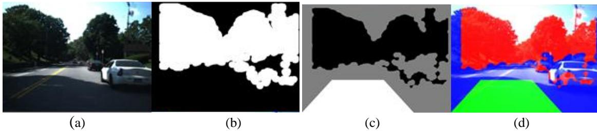
Fig. 2. Example of training mask generation. (a) The rectified left image of the stereo input frame. (b) The obstacle map (white is obstacle and black is non-obstacle) generated by the *obstacle detection* processing block. (c) The training mask containing the weak labels. In this mask black is a weak obstacle label, white is a weak road label, and gray is unknown. (d) Training mask as an overlay on the rectified left image.
