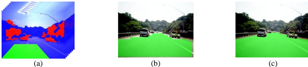
Fig. 3. The automatically obtained train mask sets (a) in which red is a weak obstacle label, green a weak road label and blue is unknown. The classification result (b) and the ground truth (c).
